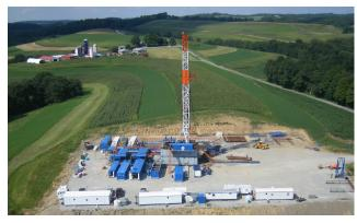
Horizontal drilling technology allows multiple wells to be drilled from a single pad, reducing the total amount of land impact and increasing the amount of energy produced.
