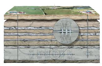
Marcellus Shale wells can be drilled both horizontally (on left) and vertically (on right). Hydraulic fracturing, a process that has been used in oil and natural gas drilling since 1949, takes place thousands of feet below the groundwater table. Every aspect of developing a natural gas well is regulated by state and federal environmental agencies.
