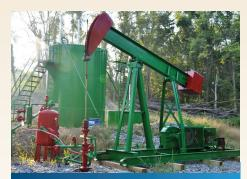
Pumpjacks like this can be found in many parts of western Pennsylvania, extracting oil from shallow geological formations. Some shallow wells produce both oil and natural gas; these wells often remain in production for decades.
